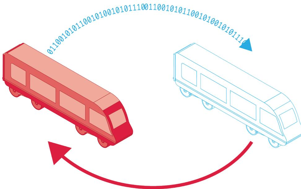
**Fig 2: A digital twin has a reciprocal relationship with its physical twin. For example, a train car may send data to a digital model of itself, while the digital twin will analyse the temperature, occupancy or performance of the car and may make positive interventions, like changing the climate controls or sending a maintenance request.**
